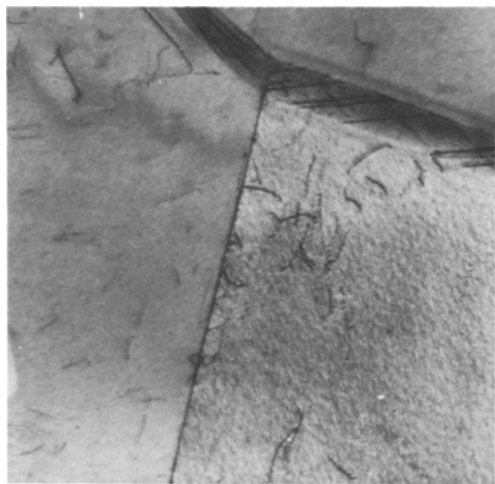
Figure 5 Transmission electron micrograph of Mn–V–C steel after solution treatment (1200°C) and brine-quenching. \times 16\,500 .
